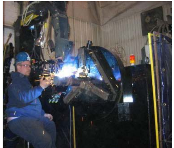
Automated welding unit at Silverado
